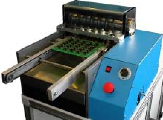
Adjustable quick change blade holder cartridge.
