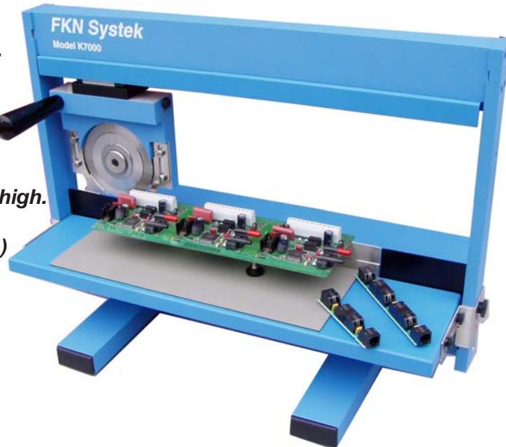
The **K7000** is a circular linear blade depanelizer developed to singulate prescored PCBs with very tight component spacing. The linear blade is 12" (304mm) long and has a .030" (.762mm) thin symmetrical cutting edge designed particularly for PCBs with closely spaced components.
