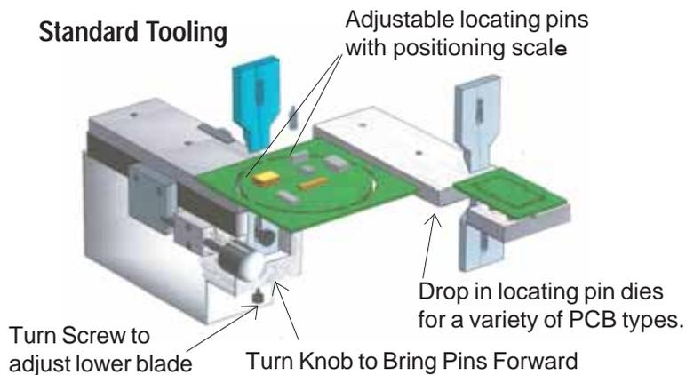
Standard tooling for the N200 is 2 blades with a guide pin die mounted on the adjustable slide block. Standard guide pins are .090" in diameter for the most popular size of routed section. Custom sizes can easily be accommodated. The bottom blade is adjustable to create a zero gap between blades.
