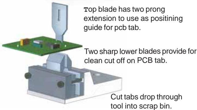
One option for separating odd shaped panels where tooling pins are difficult to place close enough together, or where the radius for singulating a panel varies depending upon the position of the tab (ie, kidney shaped or oval panels) is to use a top down punch with two sharp support knives on both sides to slice the tab from the panel to be singulated.
