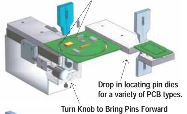
The N200 is a low cost top down air operated punch for singulating tab routed PCB panels one tab at a time. An upper and lower matching knife blade is used to pinch the tabs apart. This method produces less stress on the PCB than a punch and die since the cutting action takes place from both sides.
