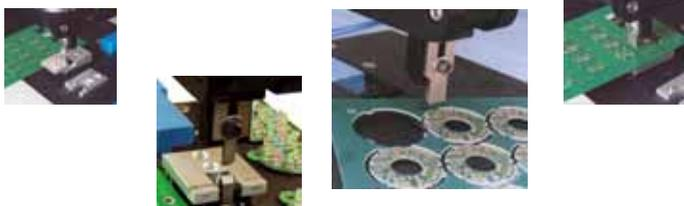
To speed up the process of singulating tab routed panels in an economical manner, it is possible to use the 4 blade die set with a sliding table. The operator places the panel onto the lower die positioning pins and brings the panel and die underneath the top die set. This actuates a pneumatic enabling switch which allows the top die to travel down when the foot pedal is activated. Once the panel is cut, it is brought back out from under the tool for removal from the die set.
