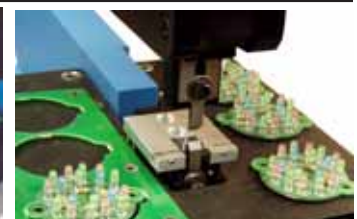
Adjustable pin locating block.
